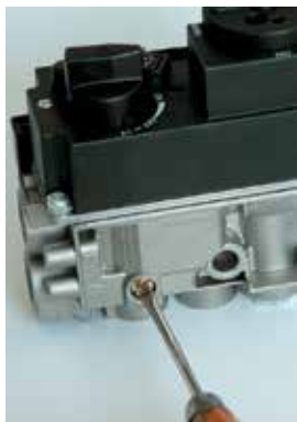
Figure 15. Adjusting method for the minimum flame height of the main burner
