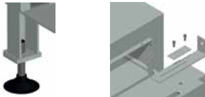
Figure 3. Levelling foot and adjustable bracket to attach to the wall
