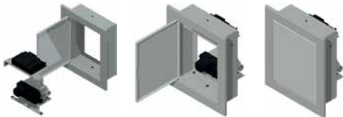
Figure 8. Mounting the gas controller with the receiver in the connection box
